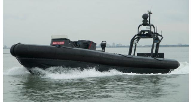
The newly designed craft, capable of 47kts and 38kts respectively, offer ship-launched manoeuvrability and promote an improved situational awareness to support the decision-making of its operators. The technology is designed to be incorporated modularly in an affordable way into the existing RIBs, such as those already used by the [Royal Navy](#).
